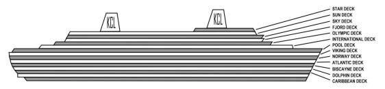
Gross Tonnage: Over 75,000. Overall Length: 1,050 feet. Beam: 110 feet. Draft: 35 feet. Engines: Parsons Turbines - 4 boilers. Cruising Speed: 25 knots maximum. Passengers: 2,000. Crew: 900.
