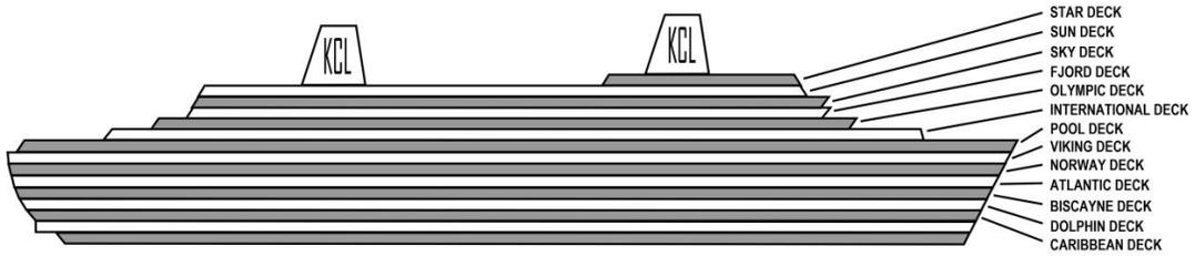
Gross Tonnage: Over 75,000. Overall Length: 1,050 feet. Beam: 110 feet. Draft: 35 feet. Engines: Parsons Turbines - 4 boilers. Cruising Speed: 25 knots maximum. Passengers: 2,000. Crew: 900.
